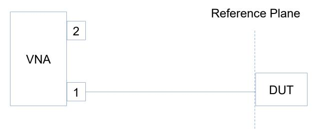
The losses in connections to the device under test must be considered as the VNA has limited output power and detector sensitivity (Dynamic Range)
